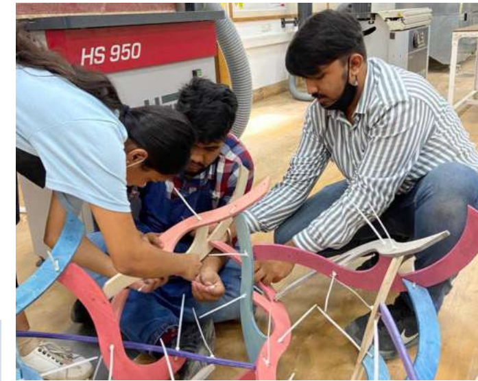
Connecting the Pieces using Plastic Zip Cables
